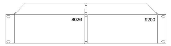
Figure 2-3. Dual Rack Mounting Option
