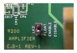
Figure 2-2. Float Enable/Disable Jumper LK2
