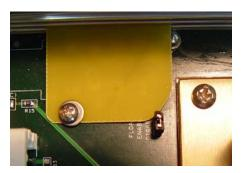
Figure 2-1. Float Enable/Disable Jumper LK1
